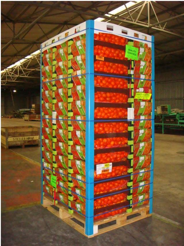
Nadorcott mandarin, traded as Clemengold®, packed using the Eco Pack System™ together with plastic corner pieces and a plastic pallet cap.
